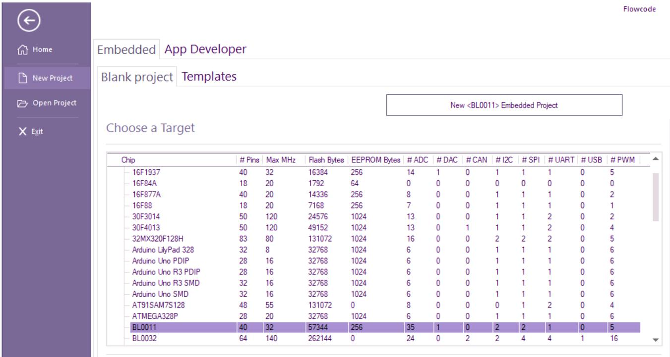
Once a new project is started, you need to select the correct microcontroller. As we are using an BL0011 board, with the default PIC16F18877 attached, we will need to ensure Flowcode has the corresponding chip selected. When using Matrix hardware, this has automatically been configured for the correct config properties and clock speed etc.
