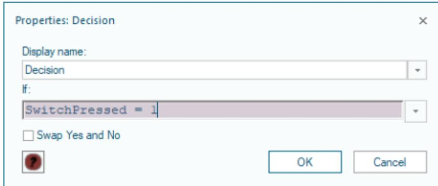
Since we are creating a latch we only want to modify the value of Flag when the switch has been pressed. Therefore, we will only place code in the 'Yes' branch of the decision. We leave the 'No' branch empty. Once the switch has been pressed we want to toggle the value of Flag from 0-1 or vice versa. Place a calculation box within the Yes branch. The statement here `Flag = !Flag` will toggle the value of Flag between 1 and 0 each time it is executed.
