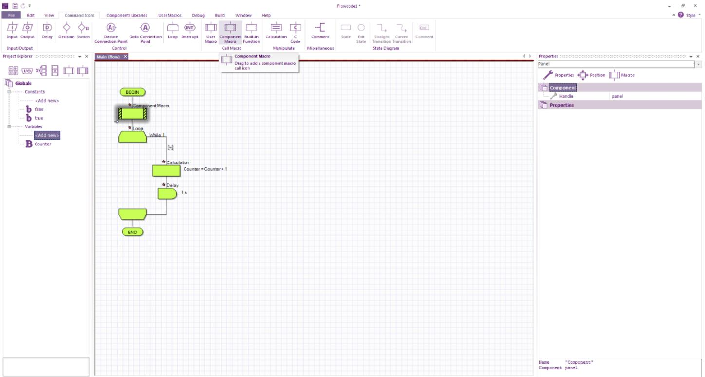
Open its configuration properties, as usual, by double clicking on the component macro. You will see the box below. Press the + button next to the LCD\_4x20 component to access the available component macros.
