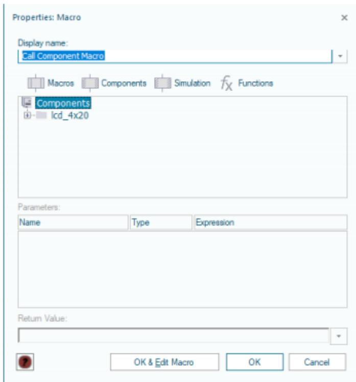
Once opened you will see a list of 13 component macros available for the LCD screen. These are all pre-written sub routines, developed by Matrix, to assist you with using the LCD screen. The first we want to use is 'Start'. Select Start and press 'OK'.
