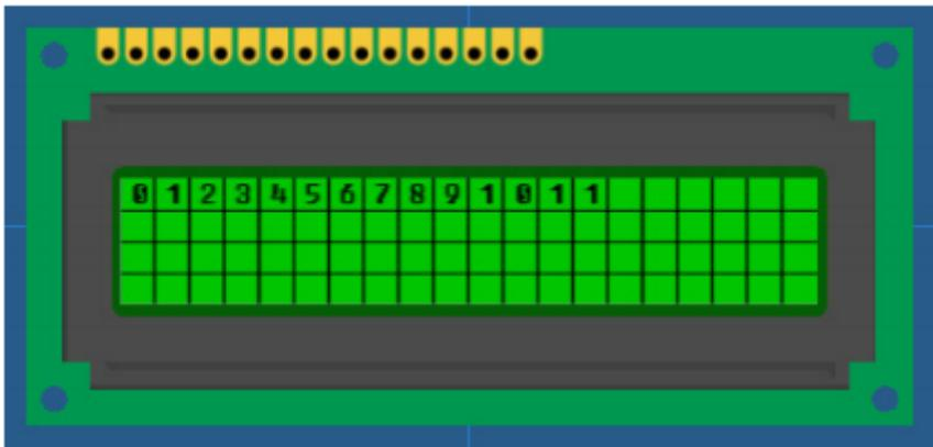
What we need to do is clear the LCD screen each time we write a new value. Luckily for us executing a clear screen routine also moves the cursor position back to (0,0). Add another component macro above the PrintNumber macro, and configure it to 'Clear'. We have now finished our third and final example. You should first test your program is right by comparing it to the code listing below. Simulate, before downloading to hardware to
